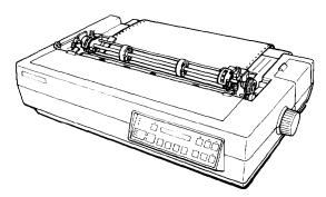
3. After the paper is loaded in the push tractor, see that the printer is off line. Press the **LOAD/EJECT** button to load the paper. Then press the **FORM FEED** button to advance the paper one page so that you can fit the paper onto the pull tractor.
